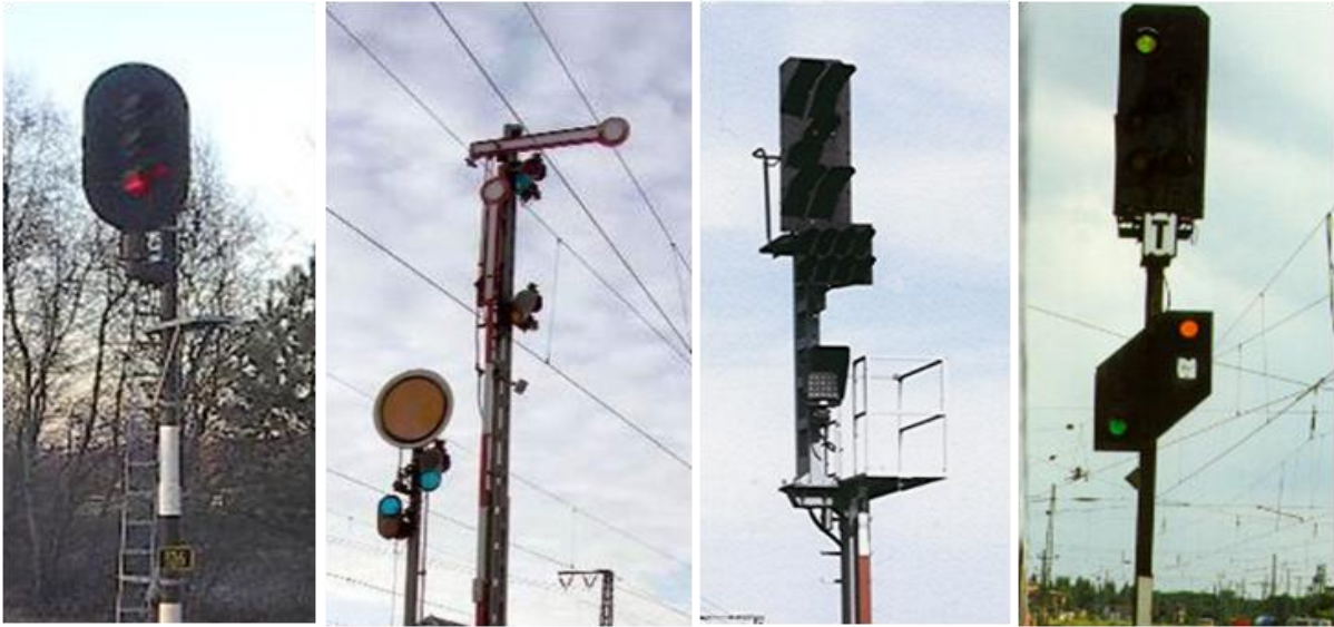
Figure 8: left to right; Dutch main signal, German mechanical main signal including prior signal, German main light signal HI- type and German light signal Ks- type including prior signal (Source: www.stellwerke.de )
